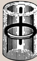
ONE STRAIGHT AND ONE CIRCULAR Used with unidirectional load, either pressure or non-pressure fed.
